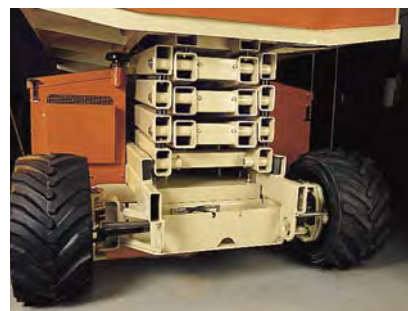
Strengthened Arm Stack for Improved Stack Rigidity
